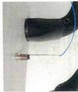
Figure 7: Correctly Positioned and Locked Fiber Optic Probe
