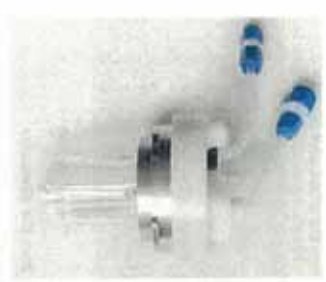
Figure 59. Fully Assembled Jacket/Attenuator
